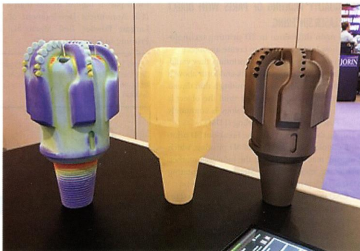
Figure 2. Printed drill bits : Colorjet Printing, Multijet Printing, and Direct Metal Printing (Titanium). 3D printing technologies manufactured three versions of this downhole drill bit. (Source: 3rd Dimension Industrial Printing).
