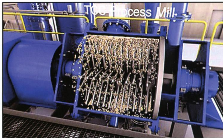
Figure 2: Cylindrical mill with hammers.
