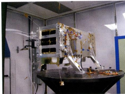
An Indian Polar launch vehicle placed the nanosatellite, about the size of a microwave oven, in orbit at an altitude of approximately 310 miles (CLAIRE's Launch, GHGSat). This 33-pound instrument orbits the earth every 90 minutes; however, any single point on the earth's surface can be measured every two weeks.
